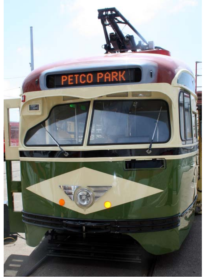
Car 529 sports a new LED destination sign as it prepares for its debut on the Silver Line.
