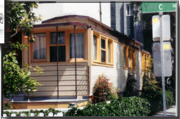
Along with the clerestory, the distinctive shapes of the original center section windows on the 1910 California car have been preserved and moved. [Photos by Chuck Bencik]
