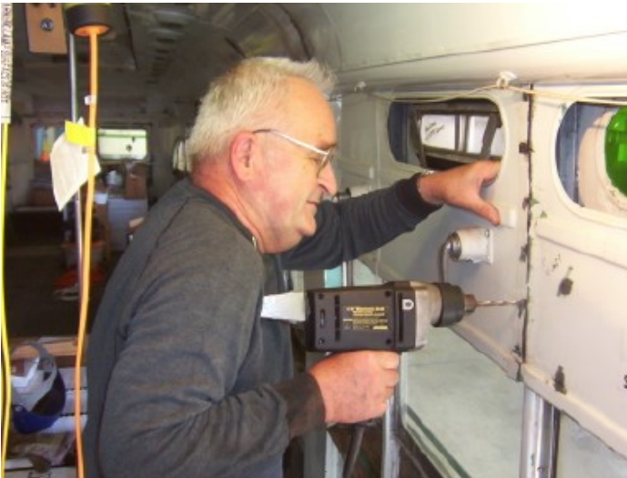
Chuck Bencik takes a drill to a stuck screw on October 10 in Car 1122. Many of these fasteners had to be removed "the hard way".
