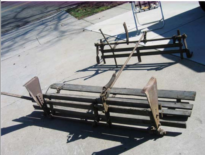
This assembled H-B Lifesaver, seen here with hanging brackets attached, was removed from PCC 1121 in Tucson.
