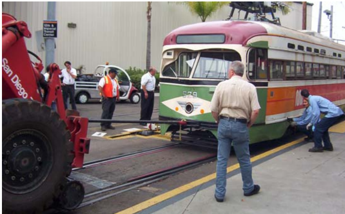
Trolley workers worked to put car #529 back on the rails after the front truck came off the track at a switch. Photo by Chris Higgins
