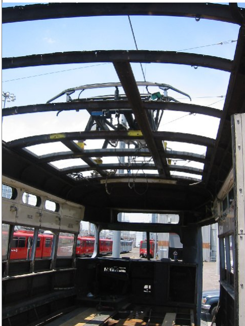
Car 529's pantograph as seen through the roof of the car. Ron Sutch photo
