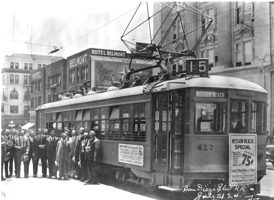
Car 417 equipped with both a trolley pole and a pantograph for use on the Mission Beach—La Jolla Line. This picture was taken at 3rd St. at Plaza on July 12, 1924. Photo from the Historical Collection - Title Insurance and Trust Company, San Diego
